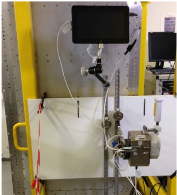
Fig. 1: The Haptics-1 Flight-spare model as set-up for crew training at the European Astronaut Centre in Germany. The system consists of the 1DOF Setup (Joystick), the touch-screen Tablet PC on a bogen arm and all periphery. Here set-up in wall-mount configuration.
