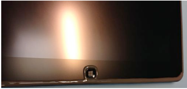
Fig. 5: Detail of application of screen protective foil to the Dell Latitude 10 tablet for flight qualification.
