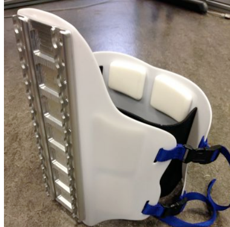
Fig. 8: Body-vest of the Haptics-1 system for experimentation in a body-grounded setup.
