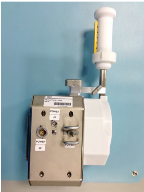
Fig. 3: Haptics-1 1DOF Setup (Joystick) including a brushless DC actuator, torque sensor and full embedded real-time computing.
