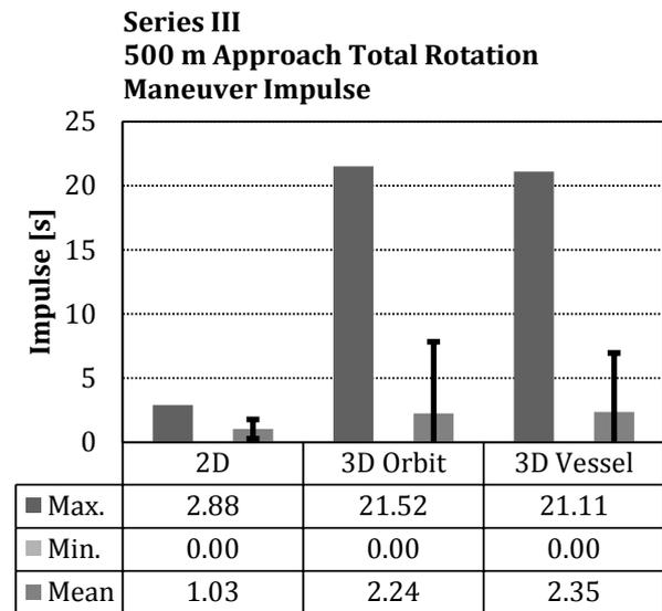
**Figure 23 - Series III: Total rotation impulse expense [s] on 500 m approach**
