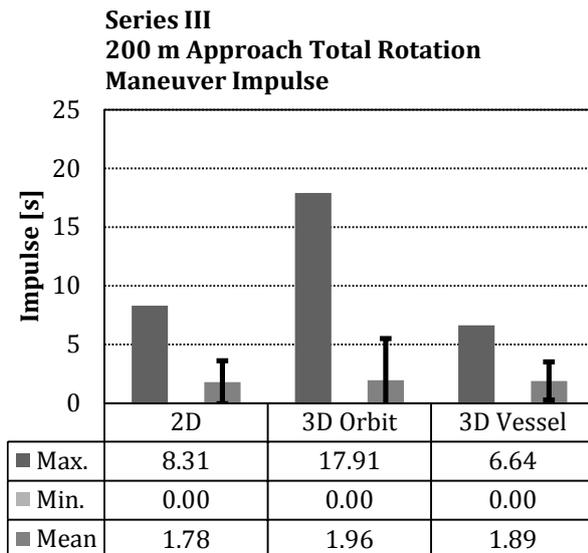
**Figure 22 - Series III: Total rotation impulse expense [s] on 200 m approach**
