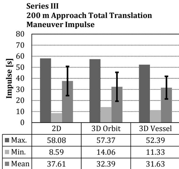
**Figure 20 - Series III: Total translation impulse expense [s] on 200 m approach**
