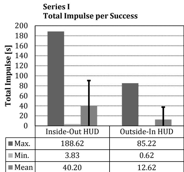
**Figure 9 – Series I: Total impulse expense [s] per successful attitude maneuver**
