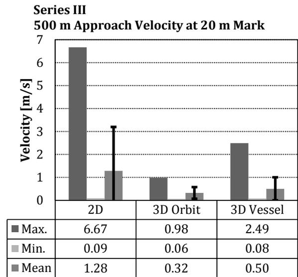
**Figure 25 – Series III: Approach velocity [m/s] at 20 m mark on 500 m approach**
