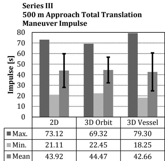
**Figure 21 - Series III: Total translation impulse expense [s] on 500 m approach**
