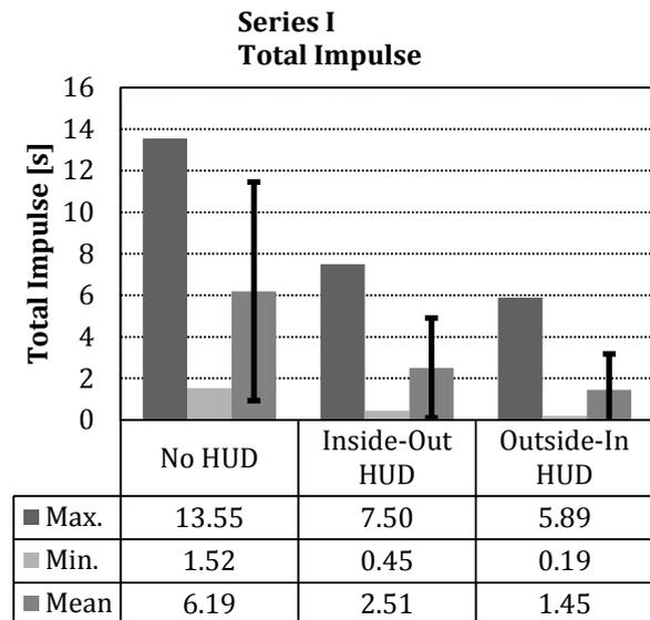
Figure 6 – Series I: Total impulse [s] required for the attitude correction maneuver
