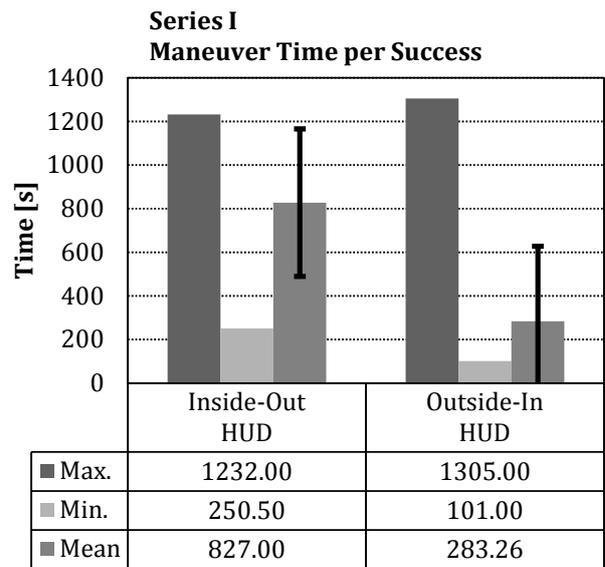
**Figure 8 – Series I: Maneuver time [s] per successful attitude maneuver**
