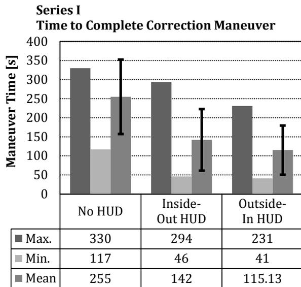
Figure 5 – Series I: Measured completion times [s] for attitude correction maneuver
