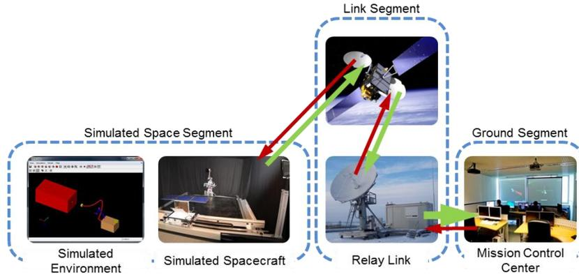
Figure 1. The components of the RACOON simulation environment.
