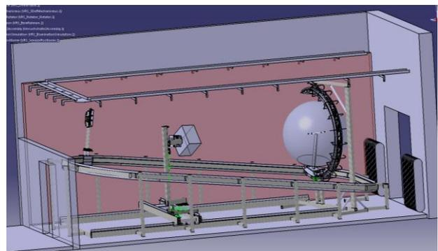
Figure 3: Future RACOON-Lab simulator full degree of freedom extension including also a dynamic lighting simulation.
