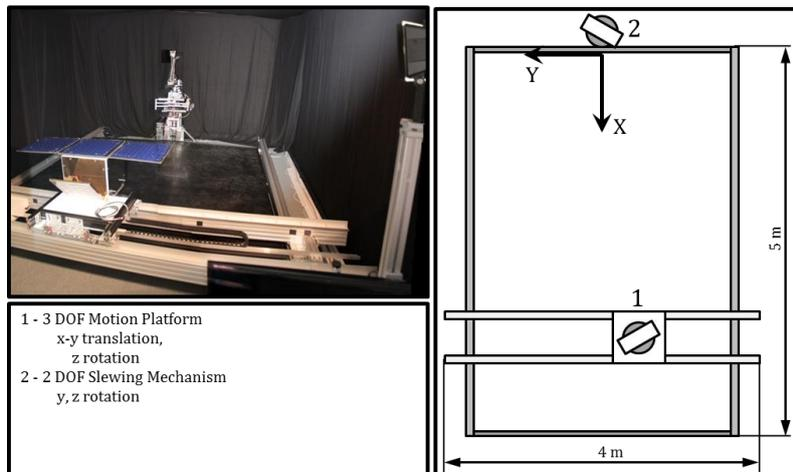
*Figure 2: Phase A Motion platform of the RACOON-Lab for simulation of OOS missions. The 2D platform has a motion envelope of 4 m x 5 m, allowing scaled simulations of close proximity operations.*
